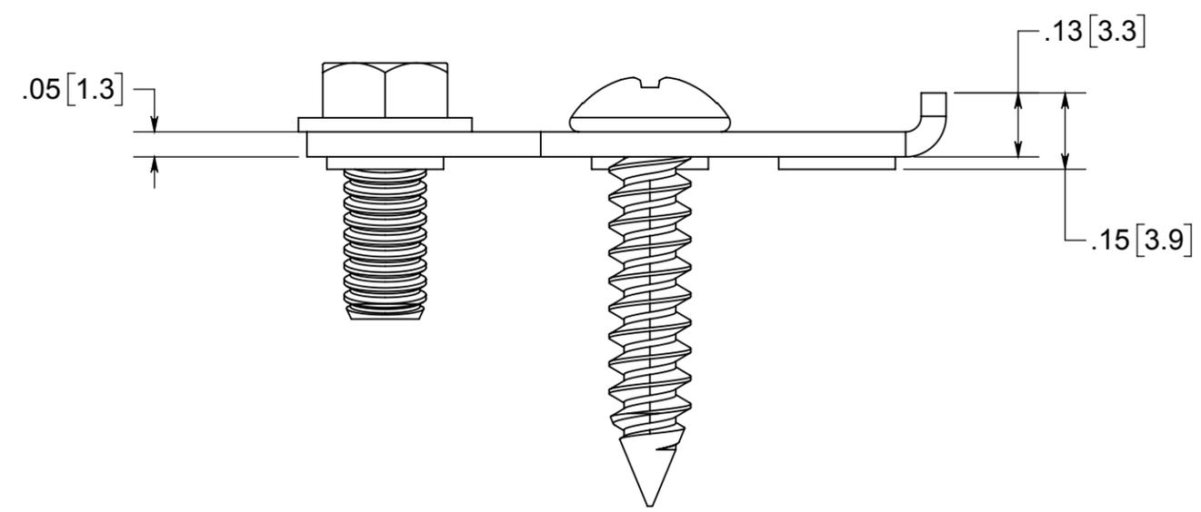
1.) GROUND STRAP MATERIAL: GALVANIZED STEEL, GROUND STRAP MOUNTING SCREW MATERIAL: ZINC PLATED STEEL, GROUND SCREW MATERIAL: GREEN ZINC PLATED STEEL
