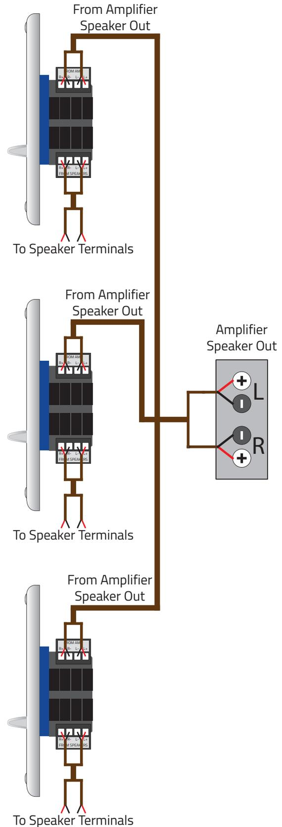
The VCSI is an automatic impedance matching volume control. Multiple VCSIs and speaker pair can be connected to an appropriately powered amplifier. There are no jumper or switch settings as long as the overall load does not exceed the amp's capability.
