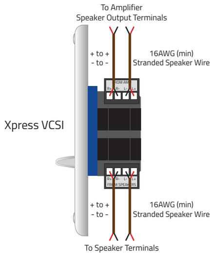
The VCSI connects with simple plug-in screw terminals. Using 16AWG (min) 2-conductor stranded speaker wire, connect the amplifier speaker OUT to 'From Amp' on the VCSI. Connect 'From Speakers' on the VCSI to the left and right +/- speaker terminals.
