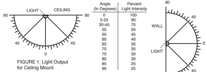
FIGURE 1: Light Output for Ceiling Mount
