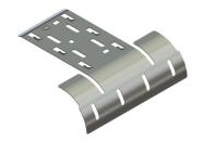
The Basic Dropout (BDO) smooths the transition of cabling dropping out of wire mesh tray. These dropouts snap into place without hardware and reduce the strain of cables as they exit or enter the tray. It mounts at the end of the wire basket cable tray parallel or perpendicular to the tray bottom.
