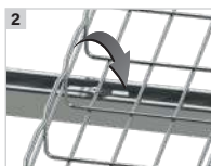
Depress FS41 and hook other side into channel support.
