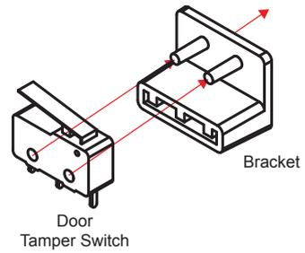
Door Tamper Switch Mounting Flange
