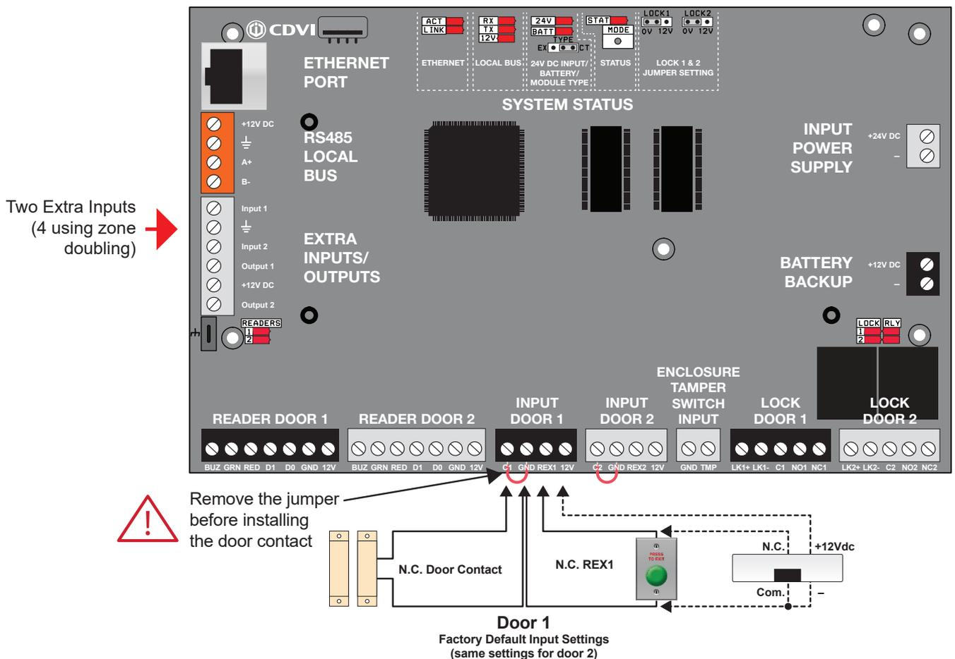
See "Recommended Wiring" section for more information on wiring type, size, and maximum length.
