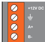
Use twisted pair wiring for RS485 connection (1 pair for ground and 1 pair for A+ B-)
