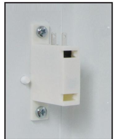
Install the door tamper switch by aligning the switch holes to the pre-installed plastic bracket pins. Press firmly to secure the tamper switch in position, then fix the bracket to its mounting flange.
