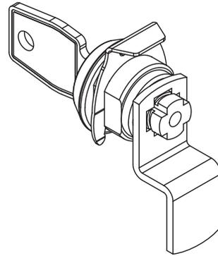
Alternatively or complementary to the box lock, the box may be secured by fixing the cover to its base using screws.
