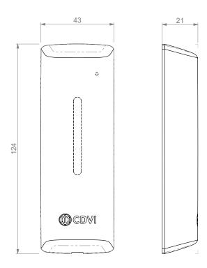
RFID Frequency band : 13,553-13,567MHz / Bluetooth Frequency band: 2,402 - 2,480 GHz Maximum transmitted power <60dB $\mu$ A/m
