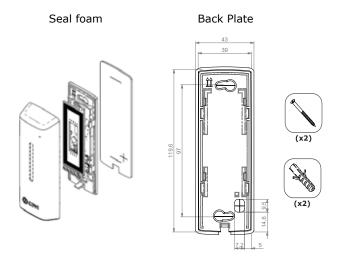
To ensure proper operation and protection of the reader, peel and stick the provided seal foam to the back of the mounting plate before installing the reader.
