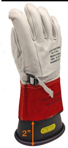
The minimum distance from the leather protector cuff to the bead of the rubber glove for this Class 2 glove is 2 inches.
