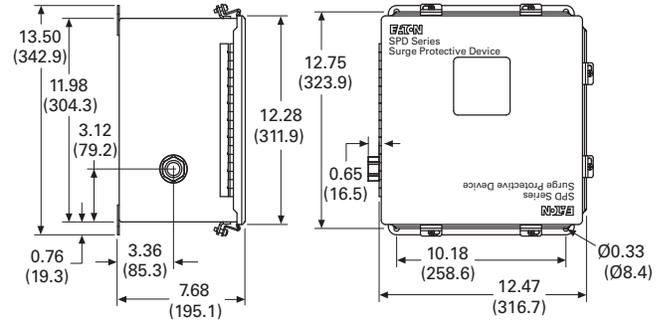
**250–400 kA Units in a NEMA 4 or 4X Rated Enclosure, Weight = 14.6 Lb**
