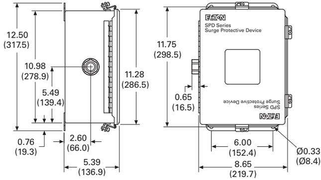
**50–400 kA Units in a NEMA 4 or 4X Rated Enclosure with Internal Disconnect, Weight = 27.5 Lb**
