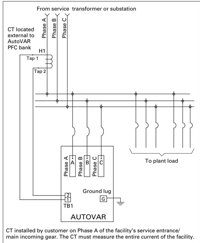
**Figure 9. Connection schematic**
