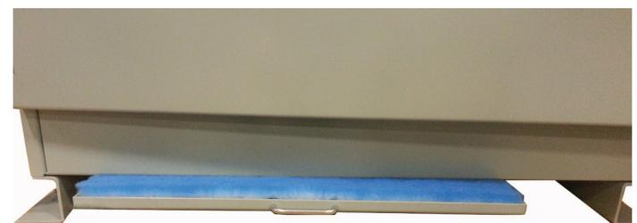
Figure 14. Dust filter location
