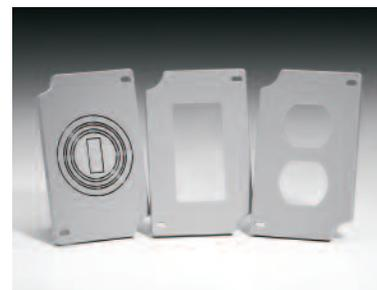
**Each Two-Gang cover** comes standard with three inserts for a total of over 60 different configurations with easy punch-outs GFCI, duplex/toggle and single receptacle toggle. Sizes of single receptacles accommodated range from 1.25" to 1.75".
