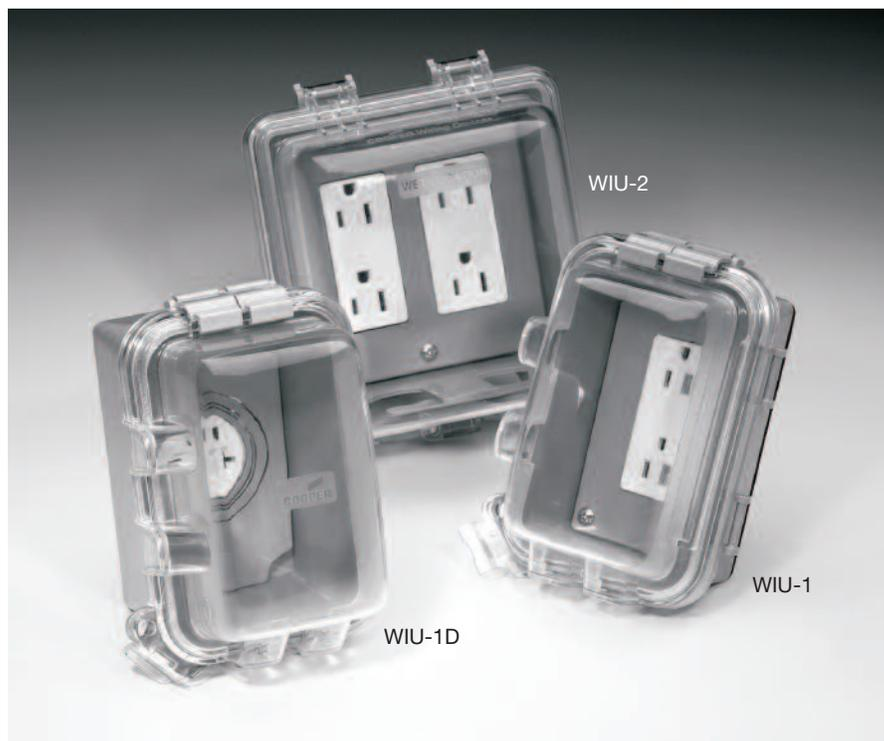
**Each Single-Gang and Extra Deep cover** comes standard with three inserts for a total of 16 different configurations. Included are duplex and decorator inserts, plus a single receptacle/toggle insert with easy punch-outs that can accommodate 5 sizes of receptacles from 1.25" to 2.125".
