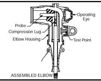
Caution: If test point cap is not installed, lubricate cap and test point and install cap.
