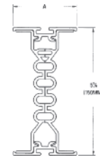
Linear Lengths Plug-in and Feeder, one bar per phase.
