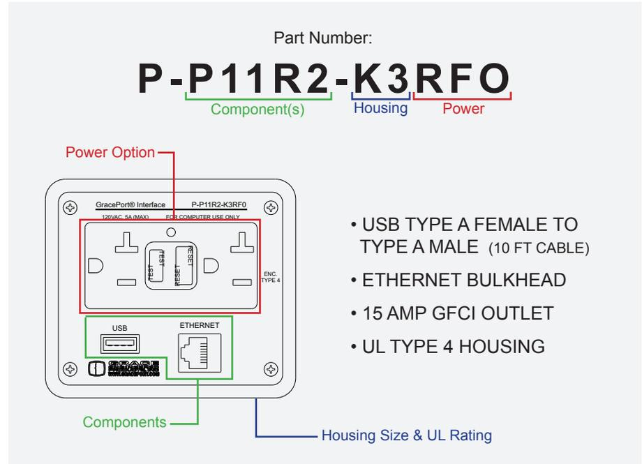
GracePorts® are fully customizable panel interface connectors that allow workers to access control panels safely and conveniently through closed doors thereby reducing the risk of arc flash. These ports can be conveniently installed on the cabinet door without voiding the UL rating of the cabinet. They can be used to program PLCs and Variable Frequency Drives (VFDs), machine interfaces, connecting laptop from outside to access and program control components.
