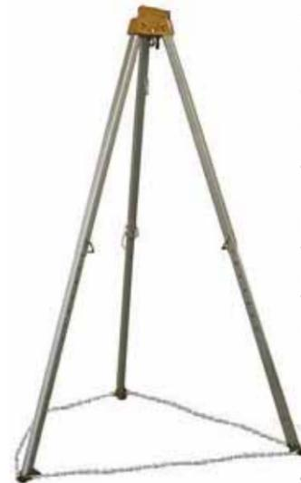
Portable fully adjustable anchorage system. The aluminium legs are made of square tubing for added lightness and required strength. The cast alloy head had an integrated pully wheel allowing a cable from a device to pass through the center of the head.
