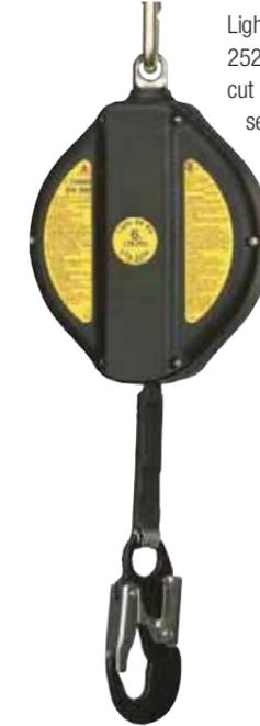
Lightweight block (only 2525 gram!) With 6 meter cut resistant Dyneema self retracting webbing and internal shock-absorber. Plastic housing with aluminium double action snap hook. The unit is completely serviceable!
