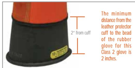
The minimum distance from the leather protector cuff to the bead of the rubber glove for this Class 2 glove is 2 inches.
