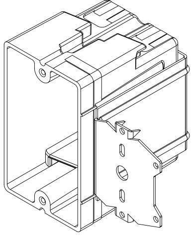
NOTES: 1.) BOX MATERIAL: FIBERGLASS REINFORCED POLYESTER, BRACKET MATERIAL: GALVANIZED
