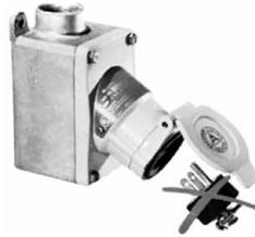
**Plug mechanical cable clamps** on the plug prevent strain on cables and meet or exceed UL 150 lb. strain relief pull-out test for classified locations.
