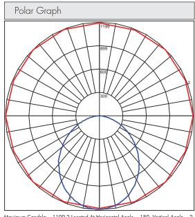
$\label{eq:maximum Candela = 1199.2 located At Horizontal Angle = 180, Vertical Angle = 2 \ \#\ 1 \cdot Vertical Plane Through Horizontal Angles (180 - 0) [Through Max. Cd.] \ \#\ 2 \cdot Horizontal Cone Through Vertical Angle (2) [Through Max. Cd.) }$
