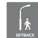
**Setback** - Automatically turns lights down to a reduced level after all occupants leave the area
