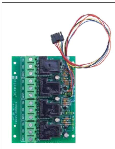
The ET9250 Relay Module can be used as a replacement part or for upgrading the number of circuits in the ET90000 controller. The relay module comes in 4-circuit packs for upgrading to a maximum of 16 circuits. Each module includes four SPDT 30 Amp relays, to be used with ET90415CR, ET90815CR, ET91215CR, and ET91615CR.
