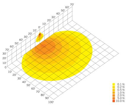
Ground mounted at 6" above ground, 10° above horizontal, shining towards building exterior wall at 28' away
