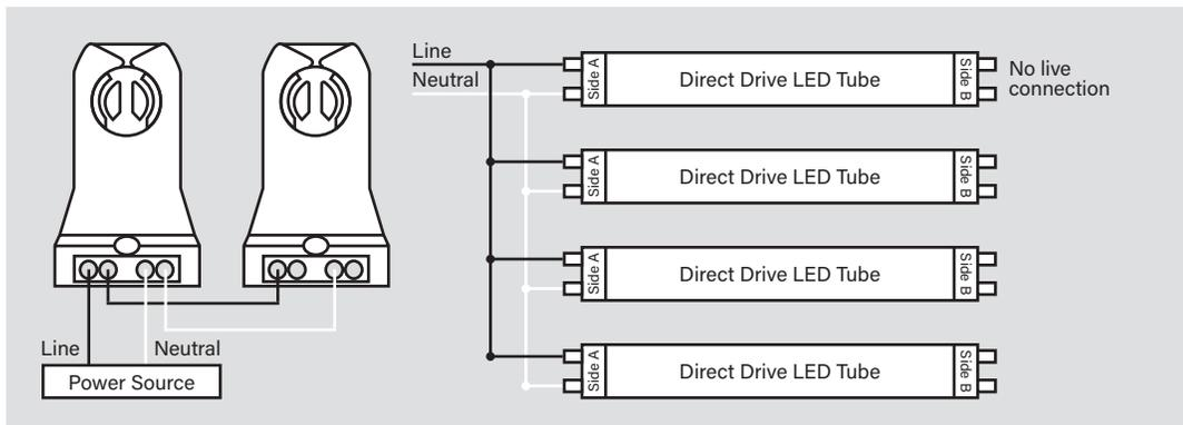
Do not install product in a fixture with shunted lampholders (found in all fixtures using instant start ballasts). If the current lampholders are shunted, remove them and replace them with non-shunted lampholders. Make new connections directly to terminals as indicated in wiring diagrams.
