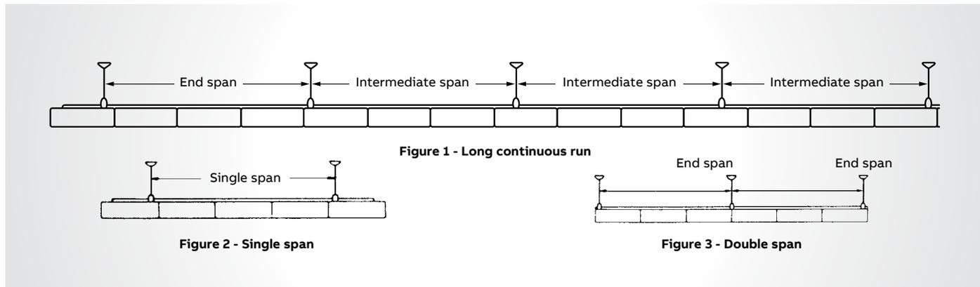
The hanger spacing is often determined by the type of building construction. The deflection then will determine the proper channel since this deflection should not exceed  $\frac{1}{240}$  of the span.
