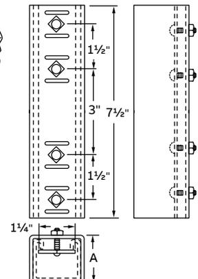
Nuts included. 14 ga steel. UL Listed for raceway. Galv-Krom® finish.
