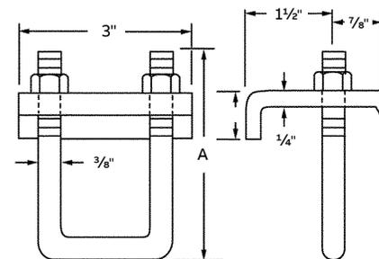
\* Load rating of 2,200 lbs. with a safety factor of 3. 3/4" steel, 3/8-inch U-bolt. Standard finish: Galv-Krom®.
