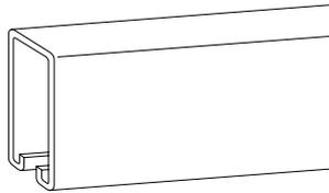
Connection by means of continuous slot.
