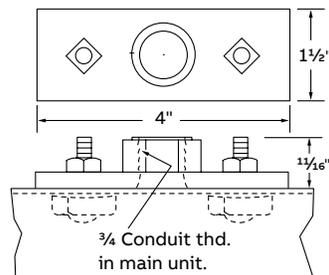
Load rating of 1,000 lbs. with a safety factor of 3. UL Listed for raceway.
