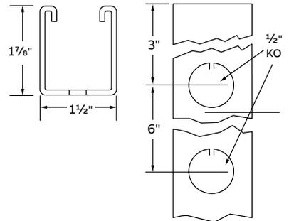
UL Listed for raceway. ½" knockouts on 6" centers. Standard finish: Galv-Krom®.
