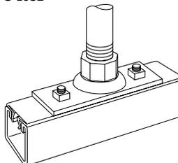
Provides a 15° swivel action (to offset possible movement) for connection of ½" or ¾" conduit to raceway channels. May be accepted for use with ¾" fixture stem when specified. Order two G-974 ¾" fasteners for channel mounting.
