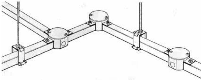
The Kindorf® Channel system serves both as a raceway for electrical conductors and a support system for the electrical outlets or tap-offs. Kindorf® is a complete wiring and support system with fittings and accessories for the design and installation of your electrical system.
