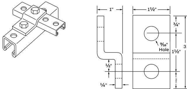
For use with B-906 or B-907 channel only. 1/4" steel. 34 lbs/C.
