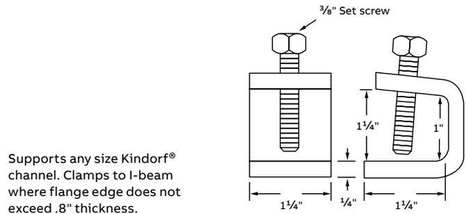
Load rating each clamp 800 lbs. with a safety factor of 3. 1/4" steel. Galv-Krom® finish.
