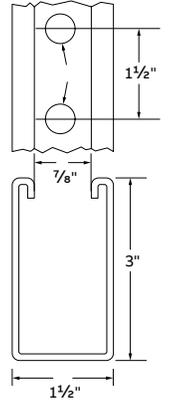
Use H-113-B bolts and B-910-1/2 steel nuts for mounting fittings. 277 lbs/C ft.
