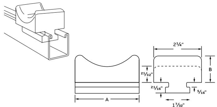
C-756-1 is for cables up to 3" O.D. Weight 72 lbs/C.
