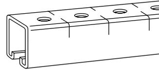
Connection by means of continuous slot or 9/16" holes on 1½" centers that match holes in B-900 series fittings.
