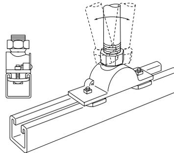
Provides a 15° swing in either direction to the channel run. Accepts ½" or ¾" conduit, or may be adapted for use with 3/8" fixture stem when specified.
