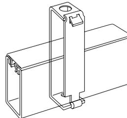
Hinged channel hanger for raceway channel.
