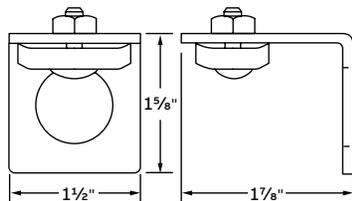
Furnished with stud nut. 12 ga steel. UL Listed for raceway.
