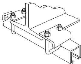
Hardened points bite into beam flange. Fits all I-beams where edge of beam flange does not exceed .8" thickness.
