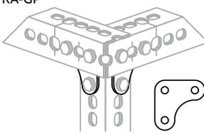
Three hole connector for extra rigid angle assembly. For use with all three types of right angle. Galvanized steel. For proper assembly, insert plate between the angle flanges for 3-bolt connection.
