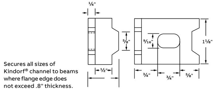
Load rating each clamp 800 lbs. with a safety factor of 3. Assembly requires one H-113-E bolt and one B-910-1/2 steel nut per clamp – order separately. 1/4" steel. Galv-Krom® finish.
