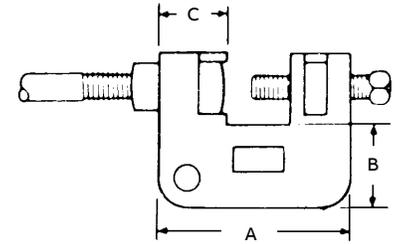
Assembly requires two H-116-C (3/8") or two H-116-D (1/2") square nuts to attach hanger rod. 3/8" steel.
