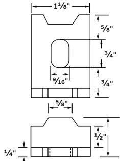
Load rating each clamp 800 lbs. with a safety factor of 3. Assembly requires one H-113-E bolt and one B-910-1/2 steel nut per clamp – order separately. 3/4" steel. Galv-Krom® finish.
