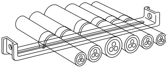
U-style channel, 12 ga steel, with Galv-Krom® finish, 3/8" turned edge. Six sizes.
