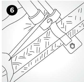
— 01 Insert pin of strap in slot of hanger.
