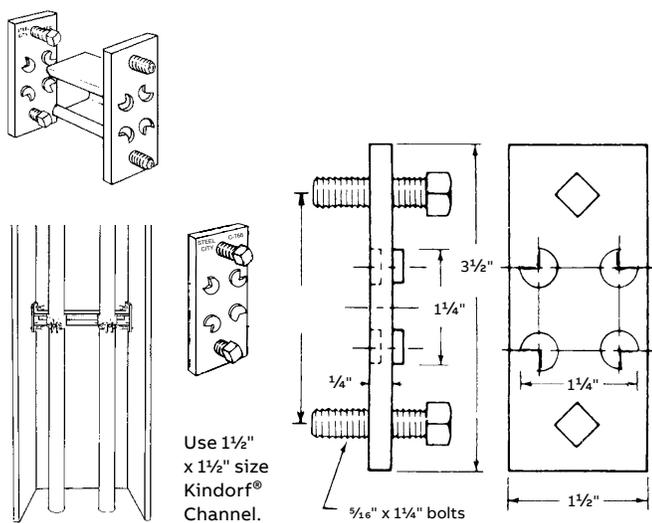
For use with 1 1/2" x 1 1/2" channel. Provides a rigid support between 'H' beam flanges for mounting pipe, conduit, outlet boxes and panel boards. Two E-768's required for installation. Use C-105, C-106 or C-107 straps for mounting 1/2" to 8" pipe on channel section. Load rating of 800# with a safety factor of 3. Galv-Krom® finish.
