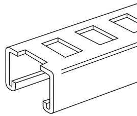
10' length slotted channel provides "cut to length" versatility. For use with standard marine steel banding. Uniformly spaced slot size 1 3/32" x 3/4" spaced on 3/4" centers. Cut anywhere along entire length.
