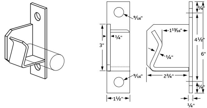
For use on storage racks constructed on Kindorf® channel. Supports reels of electrical cables, wire rope, chain and other materials. Left-hand axle support illustrated. F-736 identical except right hand. May be attached to either the continuous slot side or pre-punched holes in back or side of Kindorf® channel.
