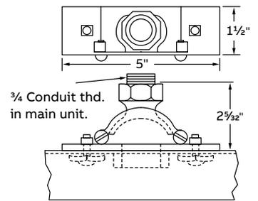
Includes two stud nuts. Malleable iron. UL Listed for raceway. Load rating of 1,300 lbs. with a safety factor of 3.
