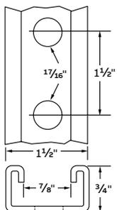
Use H-113-A bolts and B-910-1/2 or B-912-1/2 steel nuts for mounting fittings. Holes on B-900 series fittings match channel holes.
