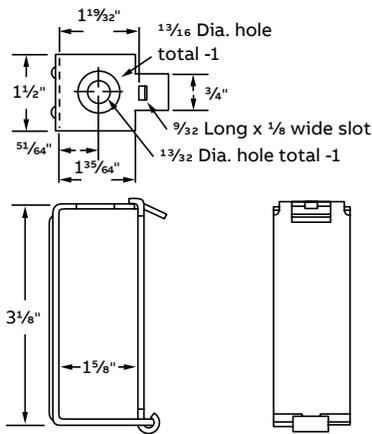
14 ga. steel. UL Listed for raceway.
