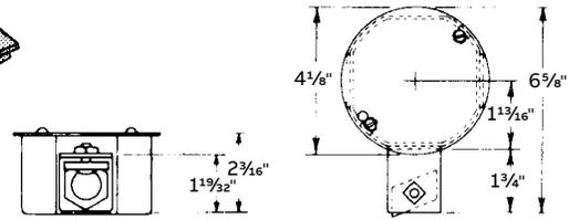
Type "E" dead end junction box for raceway channel. Accepts standard devices and covers for 4" octagon outlet boxes.
