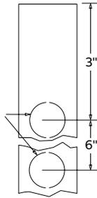
G-975: 160 lbs/C ft G-975-M: 107 lbs/C ft UL Listed for raceway. ½" knockouts on 6" centers. Standard finish: Galv-Krom®.
