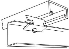
Complete with set screw for clipping a length of channel slot-side down and across the runner bars of a dropped ceiling installation.
