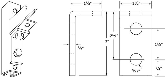
Can also be used as side-beam connector to suspend 1/2" hanger rod.
