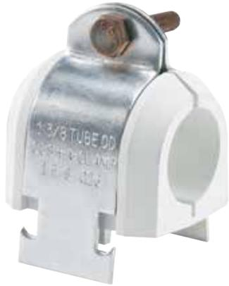
Kindorf® TPE Cable insulator clamps offer a less expensive, lighter weight and non-breakable alternative to porcelain for cable support, and they won't rot like maple clamps. The one-piece thermoplastic elastomer (TPE) insulator is flame-retardant, UV-resistant and chemical-resistant. A tapered flange isolates and protects cable. Available sizes accommodate cables from  $\frac{3}{8}$ " to  $4\frac{1}{2}$ " O.D. and fit all Kindorf® channels as well as all  $1\frac{5}{8}$ " channel systems.
