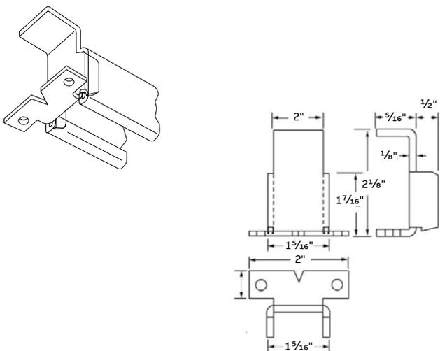
For capping the ends of D-990 continuous-slot concrete inserts. May be used on the job to make up inserts of less than 1 ft lengths of B-900 channel. Load rating of such an insert less than 1 ft long is 1,000 lbs. with a safety factor of 3. 3/8" steel. 19 lbs/C. Galv-Krom® finish.
