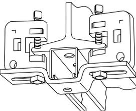
Clamps 1 1/2" x 1 1/2" Kindorf® channel to beams where beam flange does not exceed 3/4" thickness and 4" to 6 3/4" wide.
