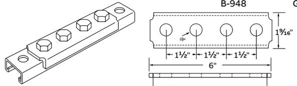
Order four B-910-1/2 nuts and four H-113-A cap screws separately. 12 ga steel. 51 lbs/C.
