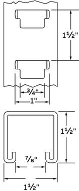
For attachment to continuous slot use H-113-B bolts and B-910-1/2 steel nuts. For attachment to T-slots use F-739 brackets 155 lbs/C ft.
