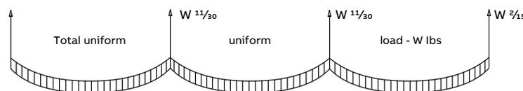
**Example** – If the total uniformly distributed load W is 1,000 lbs., the load is distributed to each support in the following manner: 133 lbs. to each end support and 367 lbs. to each inner support. Therefore, H-193-3/8, or c 'R' series hanger rod would be sufficient to support this load.
