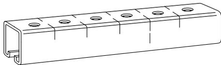
9⁄16" holes on 1½" centers punched in channel base. Connection also by means of continuous slot.
