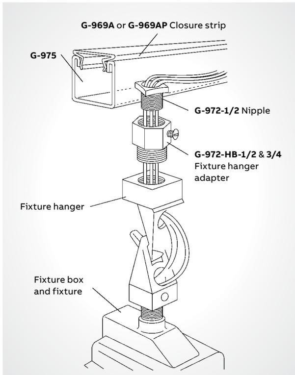
The Kindorf® Lighting Support System consists of high-quality construction materials that afford definite installation advantages to those most concerned with lighting installations. When used as a surface metal raceway, it is UL Listed and complies with National Electrical Code® Article 386.
