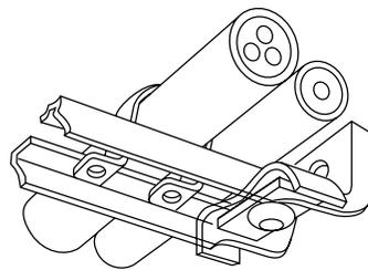
Two required for each G-1012 channel hanger to provide swivel action.
