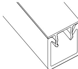
All beams should be supported in a manner to prevent rotation at supports. For beams longer than 72 inches, contact manufacturer's engineering department. Recommend sealing ends of channel with sealant after cutting.
