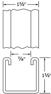
Use H-113-B bolts and B-910-1/2, B-911-1/2 or B-911-1/2-TL steel nuts for mounting fittings. 10 ft lengths only.
