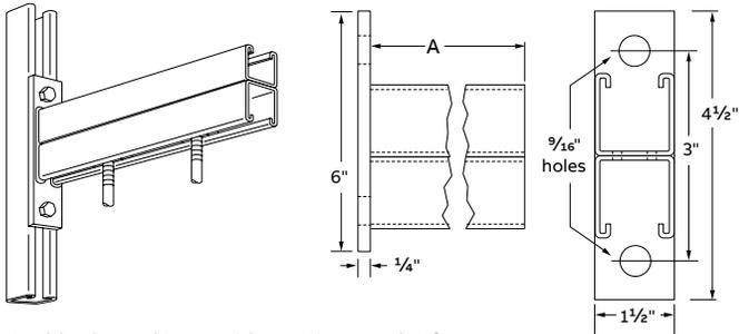
Double channel to provide continuous slot for both top and bottom mounting. 12-ga. steel, 1/4-inch back plate. May be attached to either the continuous slot side or pre-punched holes in back or side of Kindorf® channel.
