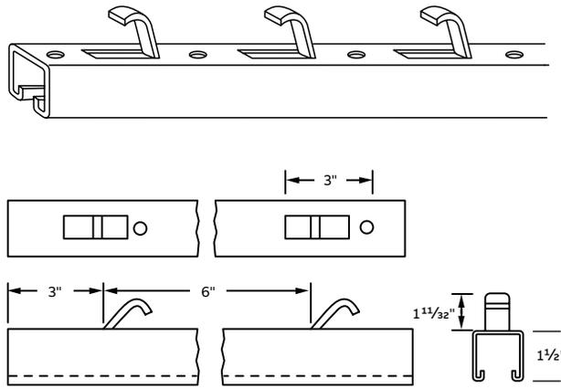
Insert is made of B-900 channel (14 ga) with anchors punched out of insert on 6" centers. Use B-910 or B-914 steel nuts for assembly. Load rating 1,500 lbs. per foot with a safety factor of 3. Available in 10 and 20 ft lengths. Galv-Krom® finish.
