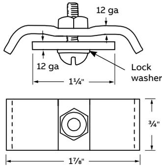
Includes 1/4" screw, nut and lock washer.
