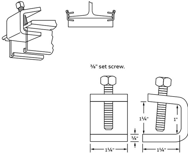
Supports any size Kindorf® channel. Clamps to I-beam where flange edge does not exceed .8" thickness. Load rating is 800 lbs. with a safety factor of 3. 1/4" steel. Galv-Krom® finish.
