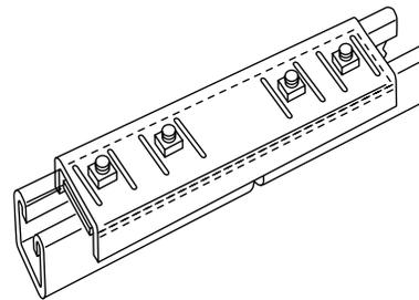
To splice lengths of raceway channel. Installed by tightening nuts on ¼" studs which are permanently attached to a smooth inner plate.
