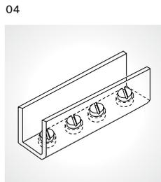
The direction-change joiner fittings for Kindorf® Channels\* expand to three, the number of channel depths available for complete raceway wiring systems. Joiner fittings are made for 1½", 1⅞" and 3" depths of 1½" wide channels.
