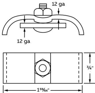
Includes 1/4" screw, nut and lock washer.
