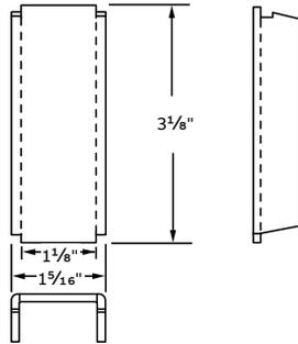
14 ga steel. UL Listed for raceway. Galv-Krom® finish.
