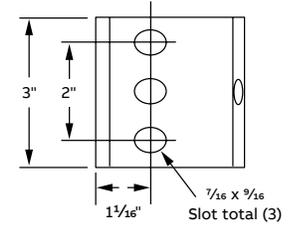
For use in attaching channel on both sides of a beam flange with slot side down. Members are shipped assembled for easy installation.
