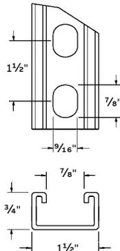
Use H-113-A bolts and B-910-1/2" or B-912-1/2" steel nuts for mounting fittings. Holes on B-900 series fittings match channel holes. Scribe marks on steel channel designate midpoint between holes for accurate field cutting. Steel 71 lbs/C ft.
