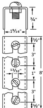
Four 3/8" x 3/4" bolts and nuts are furnished with the joiner. 14 ga steel. Galv-Krom® finish.
