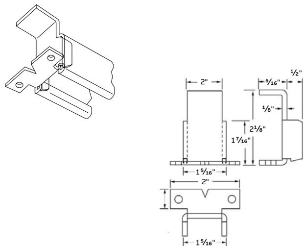
For capping the ends of D-996 continuous-slot concrete inserts. May be used on the job to make up inserts of less than 1 ft lengths of B-906 channel. Load rating of each insert less than 1 ft long is 600 lbs. with a safety factor of 3. 3/8" steel. 13 lbs/C. Galv-Krom® finish.
