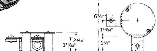
Type "L" 90° junction box for two raceway channels. Accepts standard devices and covers for 4" octagon outlet boxes.
