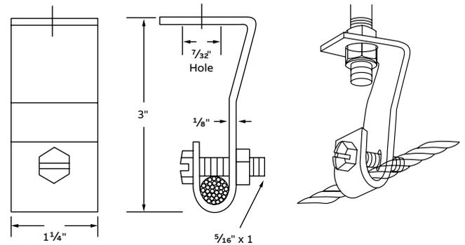
Designed for use as intermediate supports for 3/8" messenger cable. Grips cable when 5/16" screw is tightened. Provides easy vertical adjustment. Design load 1,000 lbs. Safety factor of 3. Galv-Krom® finish.
