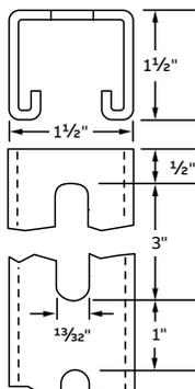
Fixtures attached to channel of G-973-2-¼ shoulder bolts. 154 lbs/C ft. 1⅜" x 3" slots on 4" centers. Standard finish: Galv-Krom®.
