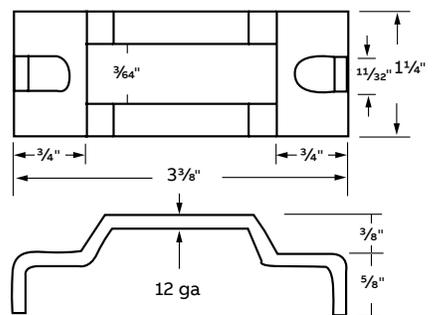
Supports one large or two small cables or tubes up to a total of  $1\frac{5}{16}$ " O.D. Both ends of hanger have nut-engaging slot.
