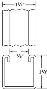
Use H-113-B bolts and B-910-1/2 or B-911-1/2 stainless steel nuts for mounting fittings. Available 20 ft lengths.
