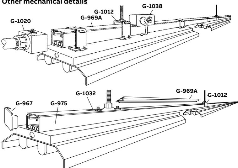
**Channel raceway system** supports and feeds fluorescent lighting fixtures.
