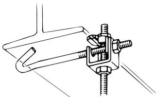
Clamps to I-beams where edge of beam flange does not exceed .8" thickness
