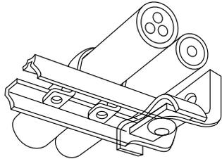
Secures single or multiple interlocked assemblies on bar hangers, mounting brackets and continuous slot channel. For installations not subject to severe shock.
