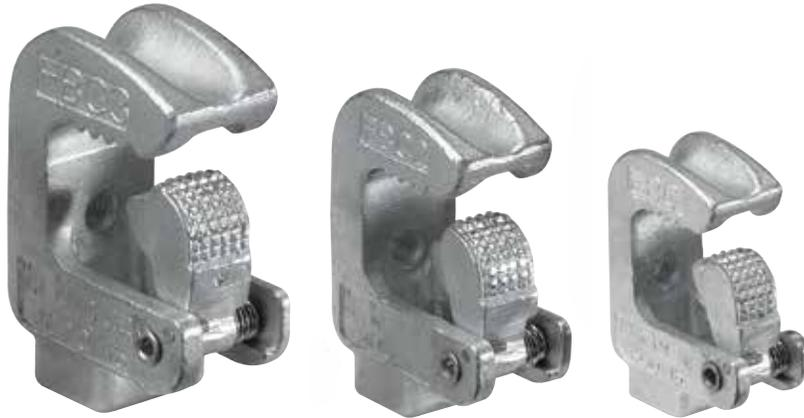
It can't get much easier than the new Kindorf® Fast Set Beam Clamp. Simply slide the clamp onto the I-beam flange, and it will remain firmly fixed while you install the threaded rod. When tightened, the threaded rod locks the tongue of the clamp against the I-beam for a fast installation and a superior hold.
