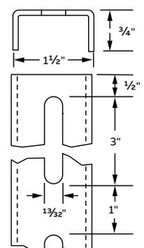
Fixtures attached to channel by means of G-973-1-1/2 shoulder bolts or G-973-2-1/4 fixture bolts. 80 lbs/C ft. 1⅜" x 3" slots on 4" centers. Standard finish: Galv-Krom®.
