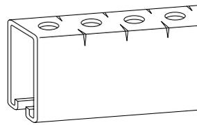
Connection by means of continuous slot or 3/16" holes on 1 1/2" centers.
