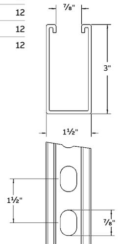
Use H-113-B bolts and B-910-1/2 steel nuts for mounting fittings. 277 lbs/C ft.
