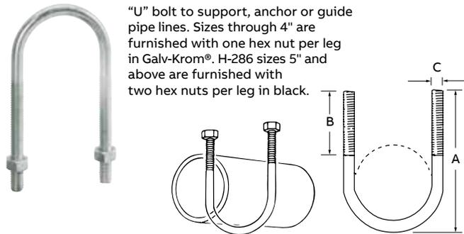
"U" bolt to support, anchor or guide pipe lines. Sizes through 4" are furnished with one hex nut per leg in Galv-Krom®. H-286 sizes 5" and above are furnished with two hex nuts per leg in black.
