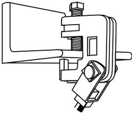
E-232 clamp with swing connector affords a convenient method of attaching to angled beams.
