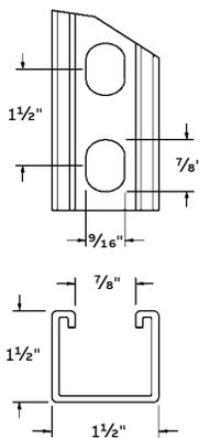
Use H-113-B bolts and B-910-1/2 or B-911-1/2 steel nuts for mounting fittings. Scribe marks designate midpoint between holes for accurate field cutting. B-905, 158 lbs/C ft. B-905-M, 102 lbs/C ft.
