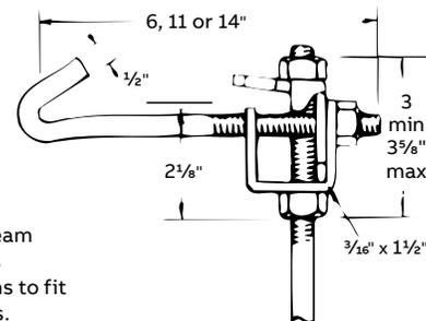
Load rating of 800 lbs. with a safety factor of 3. Assembly requires hanger rod of the proper length and size plus two H-114-D nuts. 3/16" steel, 1/2" hook rod. Galv-Krom® finish.
