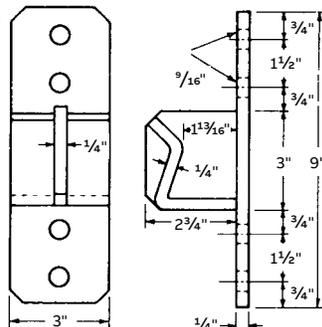
Assembly requires four B-910-1/2 steel nuts and four H-113-B bolts. To be used with F-735 and F-736. 1/4" steel. Galv-Krom® finish.
