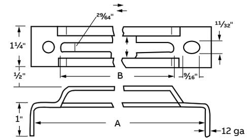
Supports cable or tube assembly, locked in place with one short  $\frac{1}{4}$ " screw and nut. Mount by welding.
