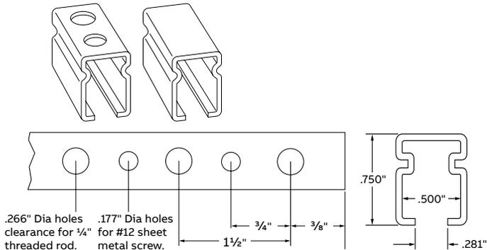
Channels are produced in 10 ft lengths. Pre-galvanized steel.
