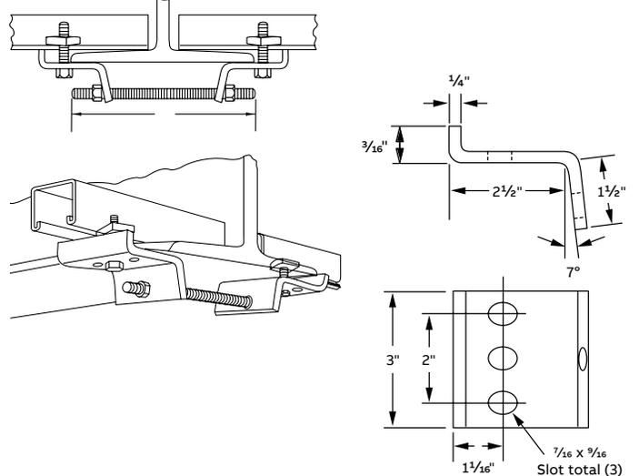
For use in attaching channel on both sides of a beam flange with slot side down. Members are shipped assembled for easy installation. Galv-Krom® finish.
