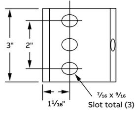
For use in attaching channel on top of beam flange with slot side down. Members are shipped assembled for easy installation.
