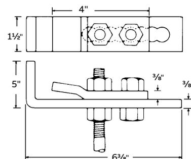
Load rating is 800 lbs. with a safety factor of 3. Assembly requires 1/2" hanger rod of the proper length plus two H-114-D nuts. 3/8" steel. Galv-Krom® finish.
