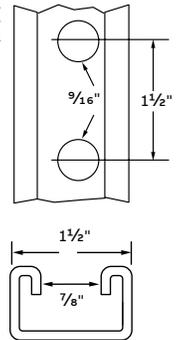
Use H-113-A bolts and B-910-1/2" or B-912-1/2" steel nuts for mounting fittings. Holes on B-900 series fittings match channel holes. Scribe marks on steel channel designate midpoint between holes for accurate field cutting. Steel 71 lbs/C ft.
