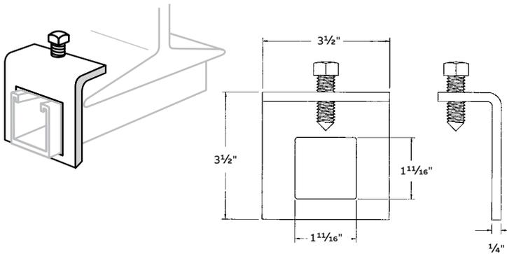
Kindorf® devices for hanging the load can deliver lower installation costs. Hanger rod and conduit pipe supports are attached to ceilings or to other structural members such as beams, columns or purlins, without drilling, welding or fastening by means of power-actuated tools. A full selection of beam clamps and hanger rod supports are offered to meet a wide variety of needs.
