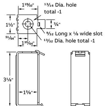
14 ga steel. UL Listed for raceway.
