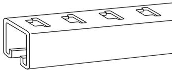
Connection by means of continuous slot or T-slots on 1½" centers in base side of channel.
