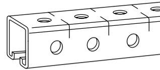
Connection by means of continuous slot or ¼" holes on 1½" centers on three sides which match holes in B-900 series fittings.
