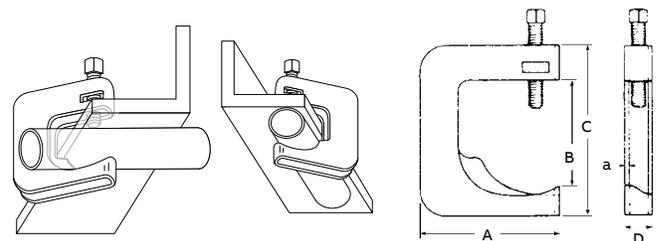
A versatile clamp for attaching conduit to any type of beam, channel, angle or column. Designed to hold the conduit snug against the support with conduit either parallel or at right angle to it. The case-hardened set screw bites into the structural member for maximum security. 1/8" steel. Galv-Krom® Finish.
