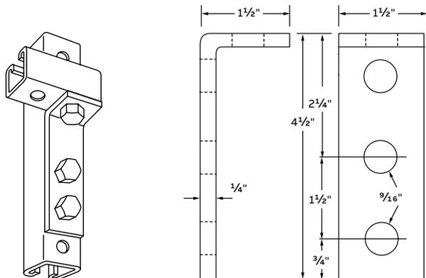
Can also be used as side-beam connector to suspend 1/2" hanger rod.
