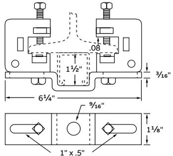
Load rating is 800 lbs. with a safety factor of 3. Furnished assembled. 1/8" steel clamps, 3/4" steel strap. Galv-Krom® finish.
