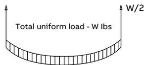
**Example** – If the total uniformly distributed load W is 1,000 lbs., each hanger must be capable of supporting half of the load or 500 lbs. Therefore, H-193-3/8 or c 'R' series hanger rod would be sufficient to support this load.
