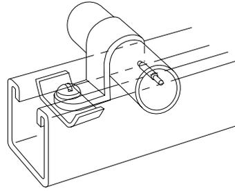
Secures single or multiple interlocked assemblies on bar hangers, mounting brackets and continuous slot channels. Designed for use with B-900 Kindorf channels.
