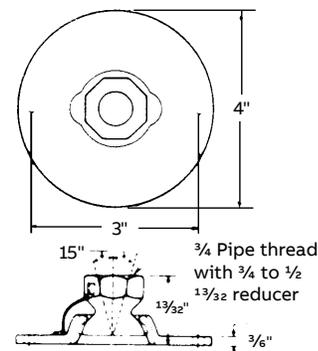
Load rating 400 lbs. with a safety factor of 3. UL Listed for raceway.
