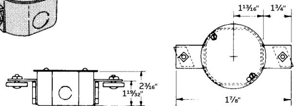
Type "C" straight through junction box for two raceway channels. Accepts standard devices and covers for 4" octagon outlet boxes.
