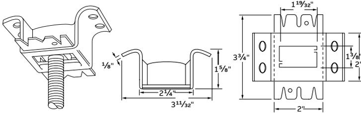
An insert with a knockout saves covering the slot or covering the opening. Load rating at 1,300 lbs. with a safety factor of 3. Accommodates hanger rod sizes from ¼" through ⅝" by means of a B-914 insert nut. ⅝" steel. 52 lbs/C. Standard finish: Galv-Krom®.
