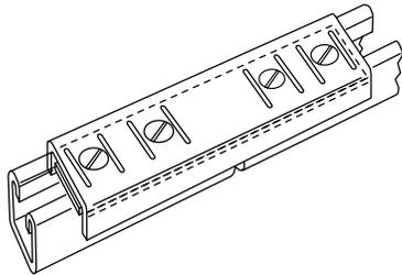
For installations where fixtures are mounted flush to slot-down channels. Fastening is accomplished by tightening flat head machine screws.
