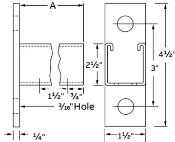
Mounts on Kindorf® channel, concrete inserts or directly to wall. Continuous-slot accepts C-105, C-106 and C-107 series pipe straps. Bracket is 12-gauge steel, 1½" x 1½" channel welded to a ¼" back plate. May be attached to either the continuous slot side or pre-punched holes in back or side of Kindorf® channel. \* Safety factor of 3. \*\* This product available in green & hot-dipped galvanized. Standard finish: Galv-Krom®.
