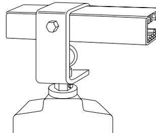
Two required for each G-1012 channel hanger to provide swivel action.
