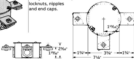
Type "T" junction box for three raceway channels. Accepts standard devices and covers for 4" octagon outlet boxes.
