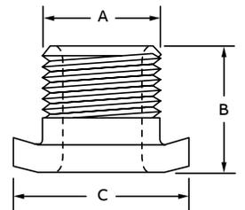
The extra length of the G-972-L-1/2 permits its use as a spacing nipple when locked into knockout or continuous slot. Load rating of 750 lbs. with a safety factor of 3.
