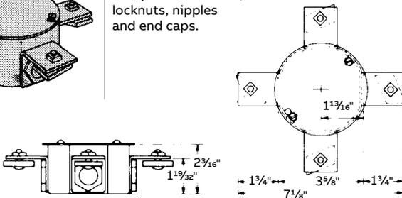
Type "X" junction box for four raceway channels. Accepts standard devices and covers for 4" octagon outlet boxes.
