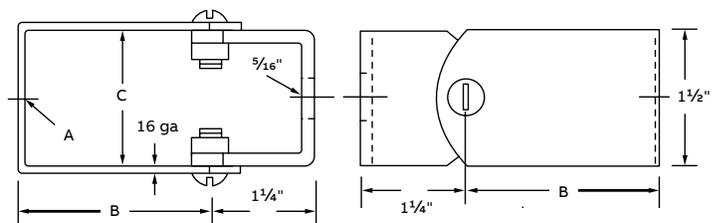
\*\* Load rating of 700 lbs. with a safety factor of 3. "B" dimension for G-962: 2 1/2"; for G-962-D: 4". UL® Listed for raceway. "C" dimension for G-962, 1 37/64", for G-962-D, 37/64". Galv-Krom® finish.
