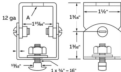
Load rating of 900 lbs. with a safety factor of 3. 48 lbs/C. Galv-Krom® finish.
