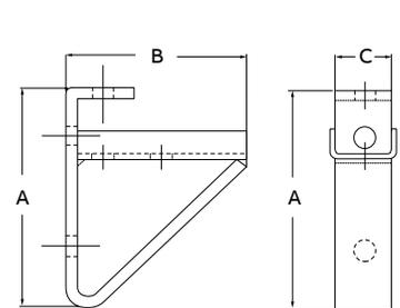
Mounts on Kindorf® channel or directly to wall. F-716-3 bracket supports 3" deep or back-to-back channels. Brackets allow for a variety of support channel lengths. The continuous tray on brackets prevent lateral movement of supported channels. Support channels can be fastened from top, bottom or both. Galv-Krom® finish.
