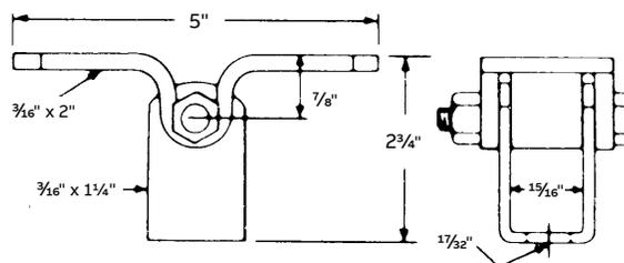
Assembly requires 3/8" or 1/2" hanger rod of proper length plus two H-114-C or H-114-D nuts. 3/16" steel. Flange has 1 3/32" diameter holes for connection to ceiling. Galv-Krom® finish.
