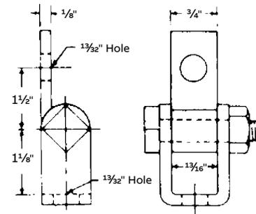
Assembly requires two (3/8") square nuts. Also screw or bolt for fastening to beam or ceiling. 1/8" steel. Load rating of 700 lbs. with a safety factor of 3. Galv-Krom® finish.
