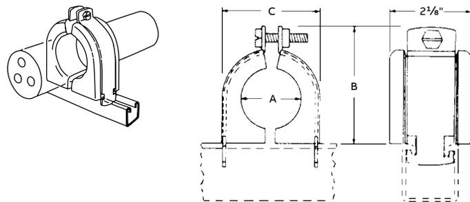
\* Also available in thermoplastic, order as C775-TP. Dry-process white-glaze porcelain insulators assembled in pairs to accept cables from 3/8" through 4 1/2" O.D. C-105 clamp with bronze slotted hex head screw and nut furnished. Fits all Kindorf® channels.
