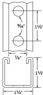
Use H-113-B bolts and B-910-1/2 or B-911-1/2 steel nuts for mounting fittings. 10 ft lengths only.
