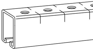
For heavier load requirements. Connection by means of continuous slot or ¼" holes on 1½" centers.
