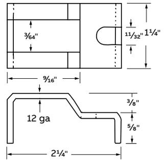
Supports one cable or tube up to  $1\frac{1}{16}$ " O.D. Strap fastens to hanger by short machine screw and nut.
