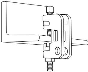
Clamps to I-beams, channels, angles and columns. Two sizes are available, one for 3/8" and the other for 1/2" hanger rod. Each takes flanges up to .8".
