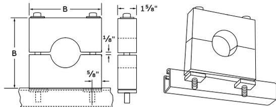
Maple blocks, impregnated with paraffin. 3/8" bolts with special nuts facilitate installation on B-900 channel. Size refers to overall dimensions of Maple Cable Clamp only. Hole will be bored to fit O.D. of cable. Orders MUST specify exact O.D. of cable. Special order.
