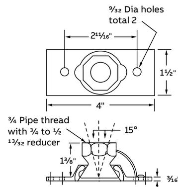
Load rating of 500 lbs. with a safety factor of 3. UL Listed for raceway.
