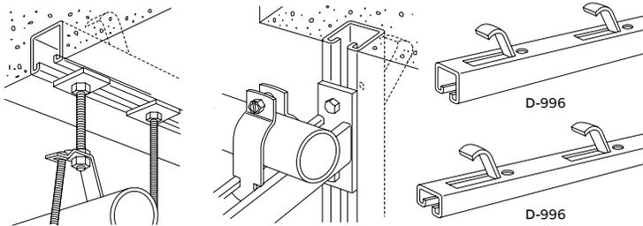
Pipe section hangs from D-990 concrete insert.
