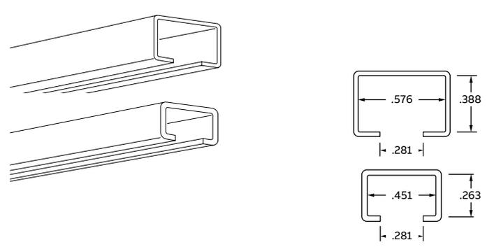
Channels are produced in 10 ft lengths. Pre-galvanized steel.
