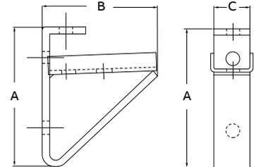
Mounts on Kindorf® channel or directly to wall. F-715 bracket supports 1½" or 1½" channels. Brackets allow for a variety of support channel lengths. The continuous tray on brackets prevent lateral movement of supported channels. Support channels can be fastened from top, bottom or both. Galv-Krom® finish.
