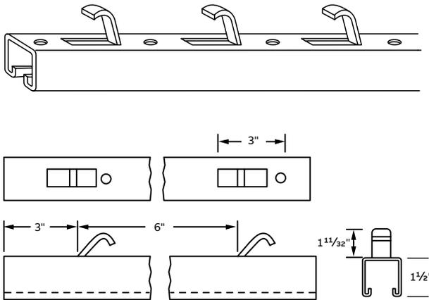
Insert is made of B-900 channel (12 ga) with anchors punched out of insert on 6" centers. Polystyrene filled. Use B-910 or B-914 steel nuts for assembly. Load rating 2,000 lbs. per foot with a safety factor of 3. Available in 10 and 20 ft lengths. Galv-Krom® finish.
