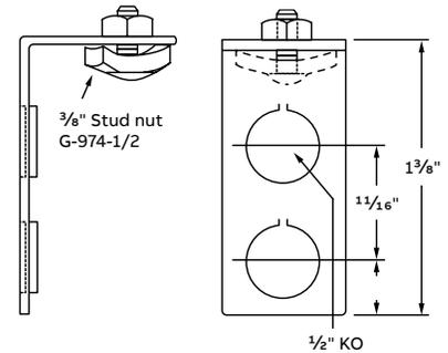
12 ga steel. UL Listed for raceway. Galv-Krom® finish.
