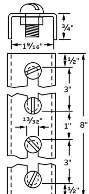
Four 3/8" x 3/4" bolts and nuts are furnished with the joiner. 14 ga steel. Galv-Krom® finish.
