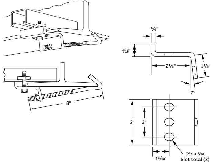
For use in attaching channel on top of beam flange with slot side down. Members are shipped assembled for easy installation. Galv-Krom® finish.
