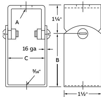
\* Load rating of 600 lbs. with a safety factor of 3. \*\* Load rating of 700 lbs. with a safety factor of 3. "B" dimension for G-962: ⅞"; for G-962-D: 4". UL Listed for raceway. "C" dimension for G-962, 1⅞", for G-962-D, ⅜". Galv-Krom® finish.
