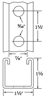
Use H-113-B bolts and B-910-1/2 or B-911-1/2 stainless steel nuts for mounting fittings. Scribe marks designate mid-point between holes for accurate field cutting. Available 20 ft lengths.
