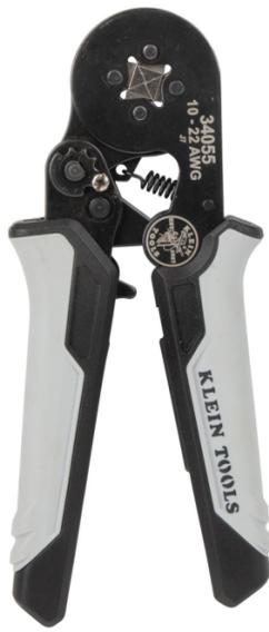
The full-cycle ratcheting ferrule crimper crimps 10-22 AWG ferrule terminals. This tool features four crimping dies that surround terminals 360 degrees for a high quality square shaped crimp. The unique design provides a low effort to crimp while maintaining a high terminal pull-off force. Built in ratchet ensures full-cycle crimping for a complete uniform crimp every time. Dual layer molded grips provide high level of comfort during use.
