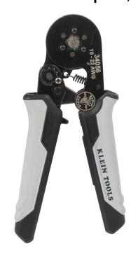
The full-cycle ratcheting ferrule crimper crimps 10-22 AWG ferrule terminals. This tool features six crimping dies that surround terminals 360 degrees for a high quality hex shaped crimp. The unique design provides a low effort to crimp while maintaining a high terminal pull-off force. Built in ratchet ensures full-cycle crimping for a complete uniform crimp every time. Dual layer molded grips provide high level of comfort during use.
