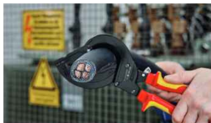
Cross-section of a steel wire armored cable
