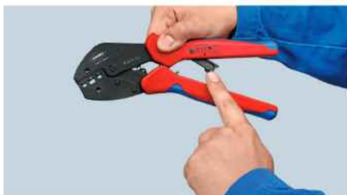
3. Fold in the service lever and press the pliers – ready for use again.
