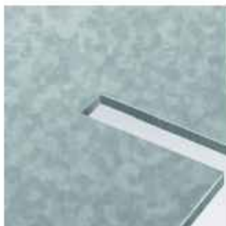
Notching and chip breaking in a single pass.
