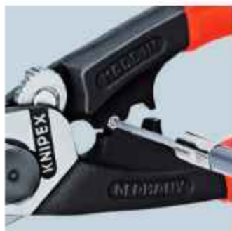
Crimping of the ferrules onto the traction cable
