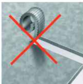
Notching without chip breaking
