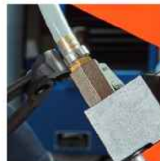
Sealing the hose connection on central lubrication
