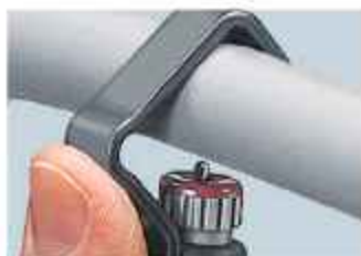
Setting the tool for circular cutting
