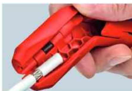
Stripping coax cable sheath
