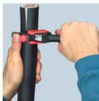
Turning the tool for circumferential cut
