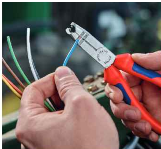
Wire stripping holes for 1.5 and 2.5 mm 2 conductors
