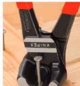
Almost flush cutting of bolts, nails, etc.
