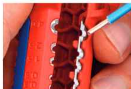
Stripping single conductor wire
