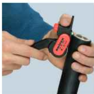
Setting the tool for longitudinal cut
