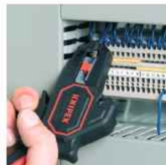
Stripping in confined areas
