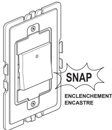
**NOTE** - If you need to remove switch after snapping into frame, first remove frame from wall box to access the three locking tabs on the back of the switch. Insert a flat screwdriver to depress tabs as you apply pressure to push switch out.
