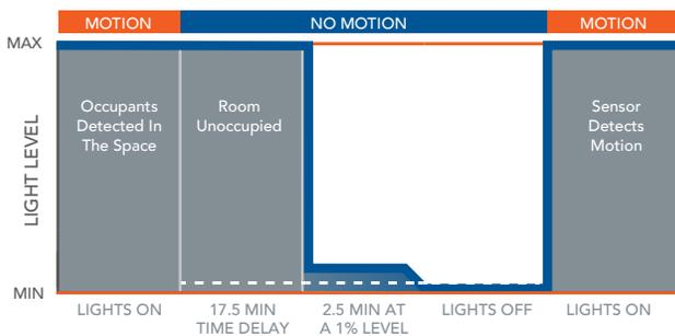
\*The presetting on the automatic dimming photocell is 5fc.
