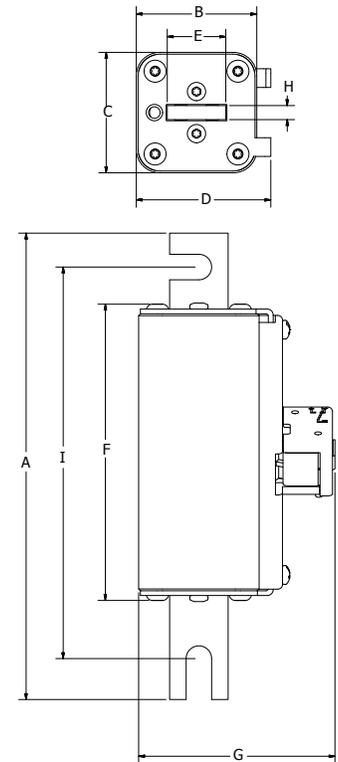
**Figure 3. DIN-blade style**
