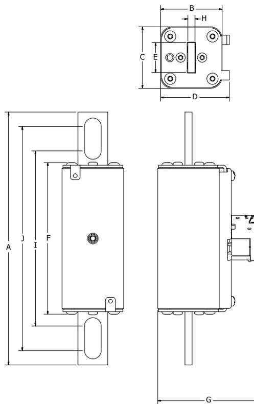
**Figure 2. Bolted-blade style**
