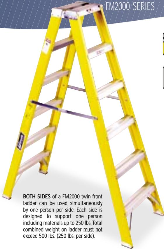
**BOTH SIDES** of a FM2000 twin front ladder can be used simultaneously by one person per side. Each side is designed to support one person including materials up to 250 lbs. Total combined weight on ladder must not exceed 500 lbs. (250 lbs. per side).
