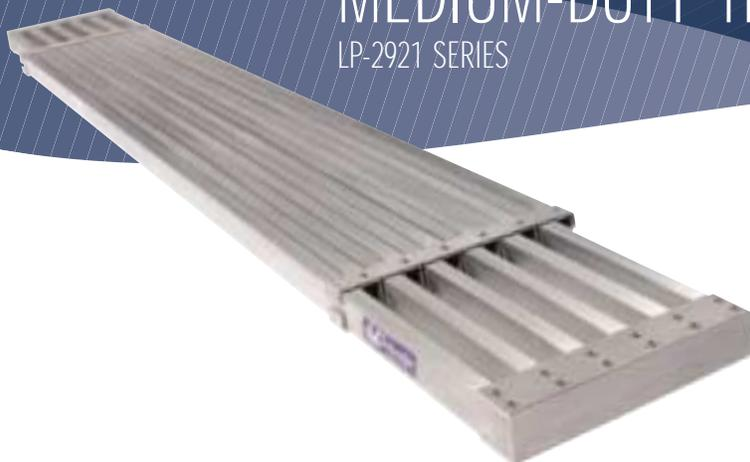
The LadderPro™ medium-duty telescoping plank is available in 9, 13, and 16-foot sizes (fully extended). The plank is manufactured with heavy wall aluminum tubing to prevent the twisting and flexing common to most other planks. The built-in, skid-resistant surface reduces slips. It stores and transports in approximately half of its fully extended length. The telescoping plank has the strength to do the job safely, and the compactness to store easily after the work is done. 250 lb. rated.
