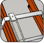
**Front-Mounted Pulley** (Fiberglass only)
