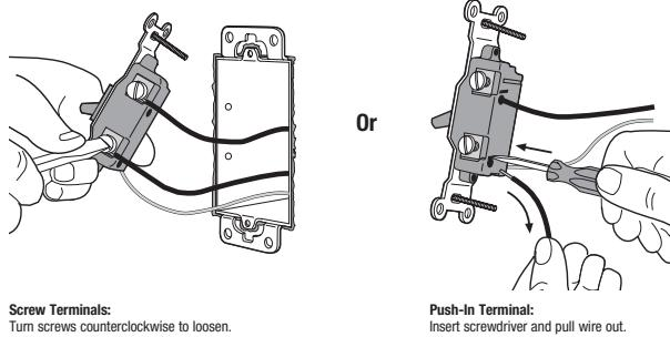
**Important Note:** Your wall switch may have two wires attached to the same screw (see illustrations below for examples). Tape these two wires together before disconnecting. When wiring, connect wires to dimmer the same way they were connected to the switch.
