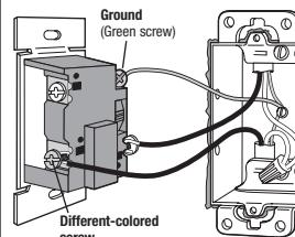
**Helpful Hint:** If you are replacing a single-pole switch with a 3-way or single-pole/3-way dimmer, the screw on the same side as the different-colored screw is not used. Tighten the screw securely.
