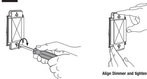
Align Dimmer and tighten screws.
