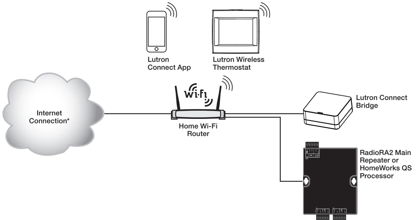
\* In order to use the Lutron App or the Lutron Connect App, a working internet connection is required to setup and control the Lutron Wireless Thermostat.
