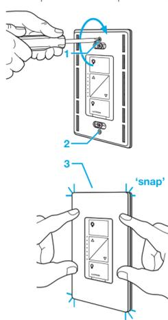
(If you installed the dimmer next to other dimmers or switches, you'll need to install a wallplate with the correct size/number of openings to accommodate all the devices.)
