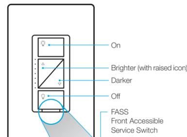
**Replacing light bulbs using FASS** Pull the FASS switch out on the in-wall dimmer to remove power at the light socket.
