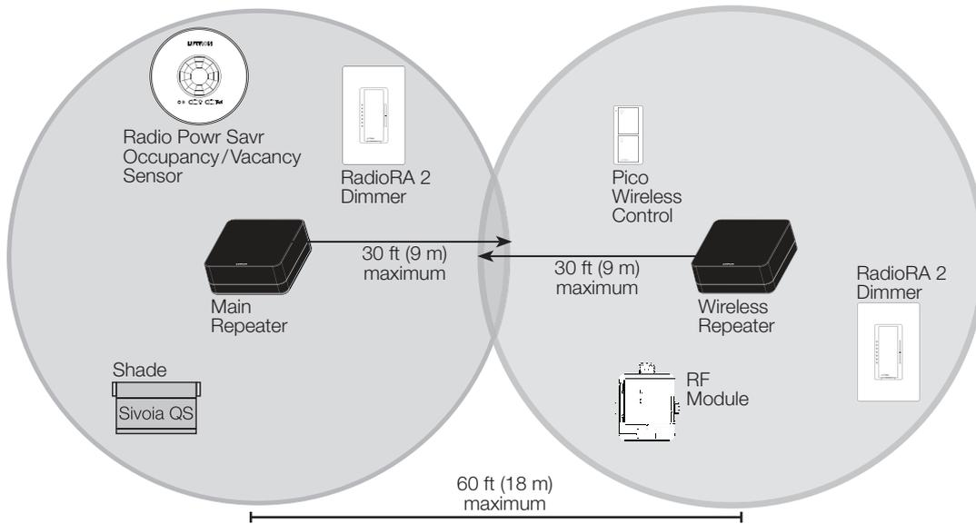
All devices must be located within 30 ft (9 m) of a repeater. The range can be extended with up to 4 Lutron wireless repeaters (L-REPPRO).
