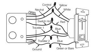
NOTE: If the SF-12P-277-3 does not turn off, or the unit does not turn on at all, the red and blue wires have been connected incorrectly. The result of the miswire depend s on the position of the other 3-way switch. Check the wiring carefully.
