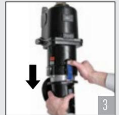
Press the pawl while withdrawing the plug from the receptacle. This is done in complete safety because the circuit is already dead.
