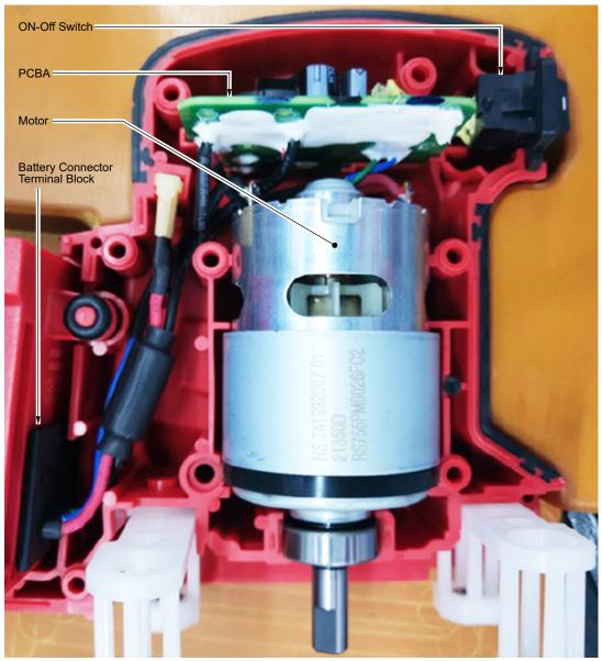
As an aid to reassembly, take notice of wire routing and position in wire guides and traps while dismantling tool.
