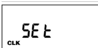
Press **HOUR** and **MIN** to advance to the present hour and minutes. Check AM/PM, and press **ENTER**.
