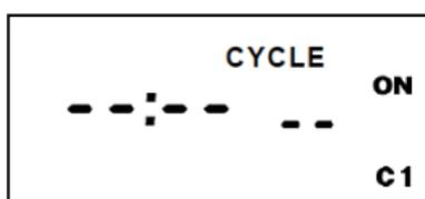
Press either **HOUR**, **MIN**, or **SEC** keys to set the desired ON duration for the cycle (ON C1).
