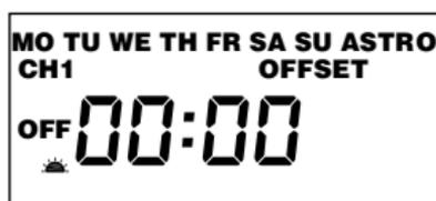
If an offset to sunrise time is required, press **HOUR** and **MIN**. Offset can be set to 3 hours and 59 minutes max. Press **EVENT** to select + or - and then press **ENTER**.
