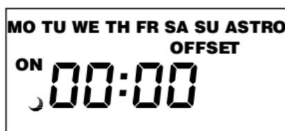
If an offset to sunset time is required, press **HOUR** and **MIN**. Offset can be set to 3 hours and 59 minutes max. Press **EVENT** to select + or - and then press **ENTER**.
