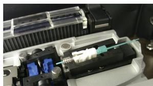
Figure 7 (Note: Remove the Extended Dust Cap Before Initiating the Fusion Splice)
