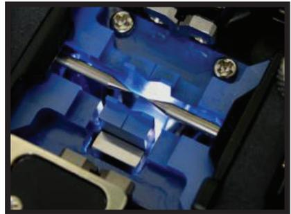
4. Using electrodes beyond 1000 arc discharges may result in greater splice loss and reduced splice strength.
