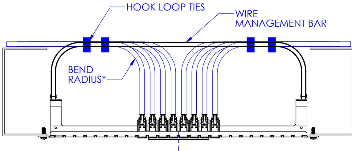
\* THE MINIMUM CABLE BEND RADIUS IS 4 TIMES THE OUTSIDE CABLE DIAMETER. HOOK LOOP TIE WRAPS SHOULD BE USED TO ATTACH THE CABLES TO THE WIRE MANAGEMENT BAR. THE CABLE AT THE EDGE OF THE PATCH PANEL SHOULD BE ATTACHED TO THE CABLE WHICH HAS ALREADY BEEN TIE WRAPPED TO THE WIRE MANAGEMENT BAR.
