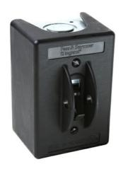
Double Pole, Single Phase AC Manual Motor Controller, suitable as Motor Disconnect - 10KA @ 600VAC, 30A max. Class J Fuse.
