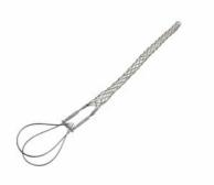
FCSD70LB: Service Drop, Closed Mesh, Locking Bale, Cable Diameter 0.70 - 0.97 inches, Bale Length 14-in, Mesh Length 9-in, Break Strength 1020 lbs.
