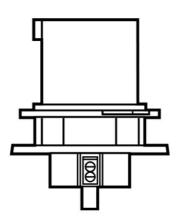
Three pole, Four wire, Pin and Sleeve Inlet. 30 amp, 3/480 volt.
