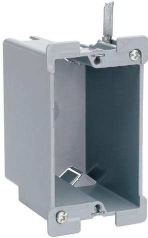
Single-Gang, Old Work Switch and Outlet Box with Swing Bracket for mounting. Adjusts from 1 1/4-inch down to 1/8-inch. Two Auto/Clamps on Each End. 100 pack.
