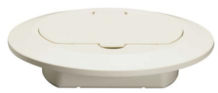
Thermoplastic Cover Includes 15A 125A Decorator receptacle, matching detachable and replacable hinged door threaded device-mounting holes drill guides for low-voltage poke-through holes accepts any Decorator device mounts on carpeting, hardwood, linoleum, tile floors Four mounting/leveling screws. .For detailed Tamper-Resistant receptacle information, visit our Tamper-Resistant Receptacles page.
