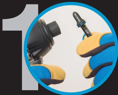
1 Choose bit size & attach it to the chuck or coupler. Fasten it well. Set power tool to MAX speed & torque if it is adjustable.
