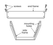
Frame construction for surface mount panels
