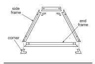
Frame construction for recessed panels
