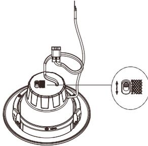
4. Plug E26 base cable connector into the LED Recessed Kit. Make sure the kit is grounded. (Fig. 4)
